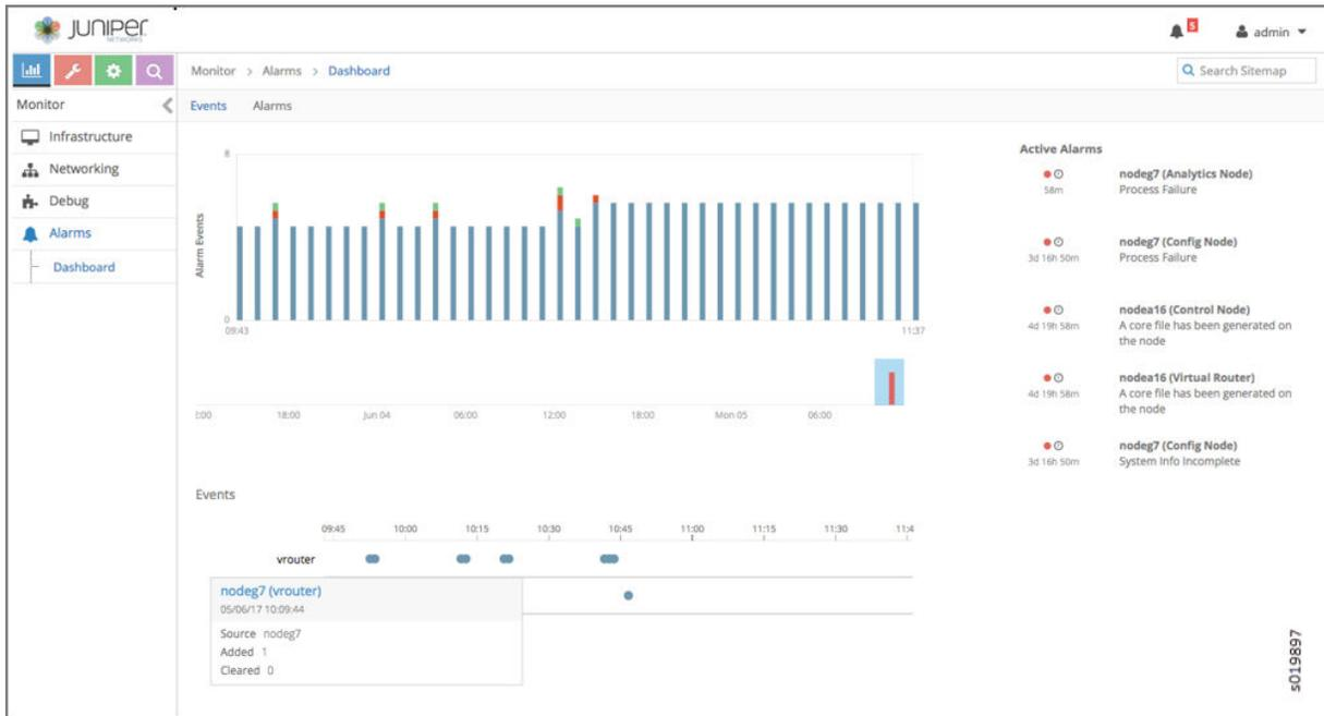
You can expand the event log in the right side panel to display a detailed event log. Click the name of any node in the list in the right panel, and the details of the current alarms are visible in the expanded view, see [Figure 17 on page 125](#).
