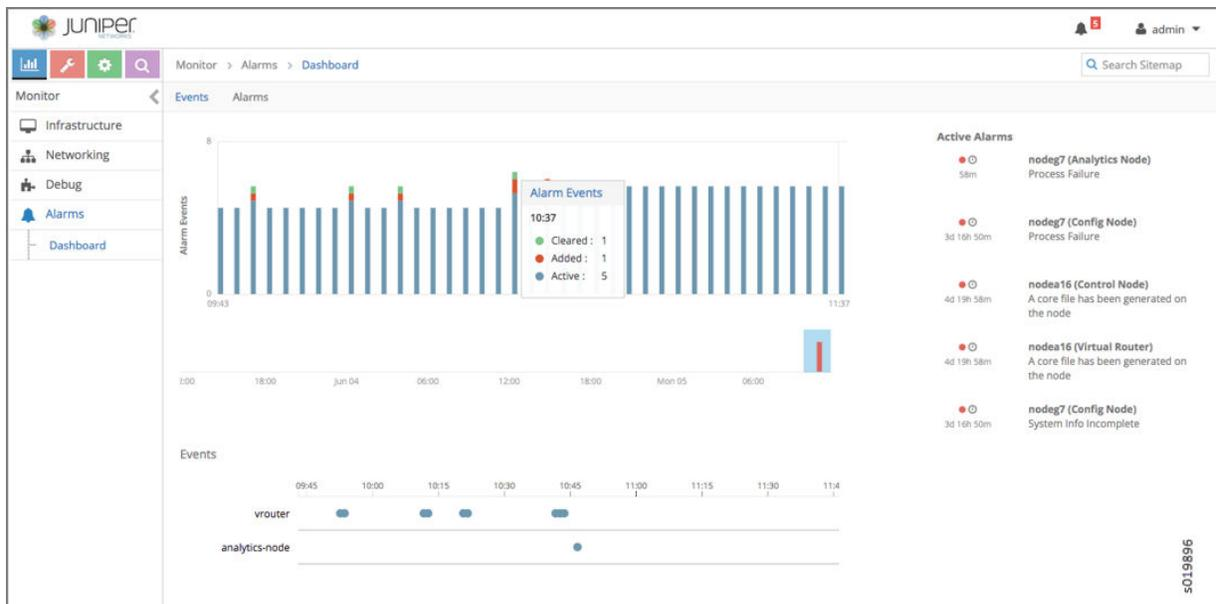
Tooltips are available on the Alarms History page. In the Events area, you can click on any node type listed to display a tooltip showing details of the events that have been added and cleared in that node, see [Figure 16 on page 124](#).
